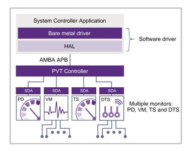
The Synopsys SLM family is designed to improve silicon health and operational metrics at every phase of the device lifecycle. SLM is built on a foundation of PVT monitor IP, data analytics and design automation. Environmental, structural and functional monitors enable deep insights from SoC manufacturing to in-field systems. Meaningful data is gathered at every opportunity for continuous analysis and actionable feedback.
