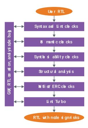
The VC SpyGlass Lint solution dramatically reduces the inherent risk in developing first-pass complex multimillion-gate, nanometer-scale SoCs by accurately detecting design issues at the RTL level. It flags almost all areas of the design that are likely to present implementation challenges.
