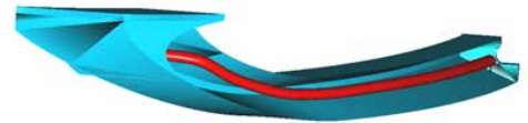
Figure 1: LED light guide daytime running light (DRL) feasibility study with luminance visualization in XYZ color rendition of the light
